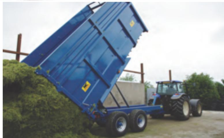
All trailers are fitted as standard with a sprung drawbar, tandem spring suspension, hydraulic brakes, handbrake, full RTA approved lights (including rear beacon) and front galvanised ladder.
