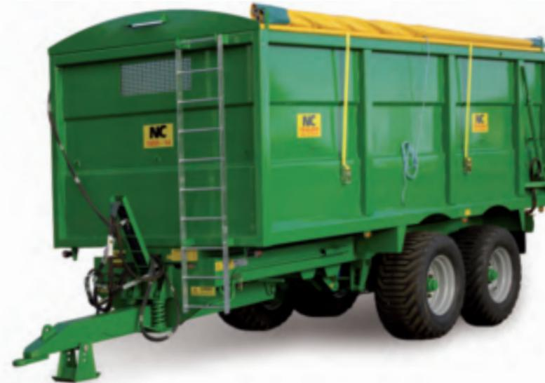
NC Engineering offer a selection of Silage/Grain trailers ranging from 10-25 Ton capacity. The monocoque body comes with a 100mm front to rear taper and tips to an angle of 50 degrees to ensure easy emptying.
