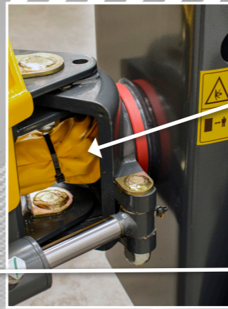
Protected hose lines
