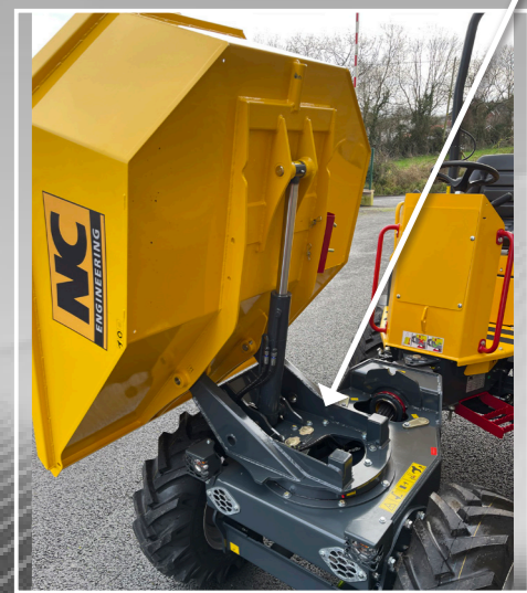
Twin cylinder power swivel 180°
