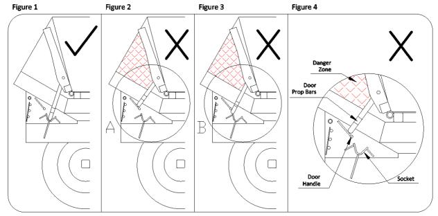
Figure 1 illustrates the door prop bars correctly engaged in the sockets.
